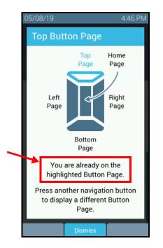
The phone will only navigate to a different page when pressing a navigation button (i.e., the page will not change without user action), and only when page navigation is allowed. In addition, the phone will return to the last-viewed page when waking from sleep, dismissing a popup, exiting a menu, and after a reboot.
