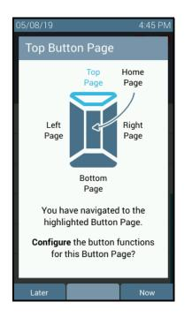
Once the phone is in button programming mode, use the navigation pad to go to any of the pages for which a button needs to be programmed (or re-programmed).
